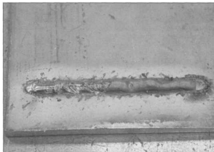
4.14 At right on this bead, you can see the dark gray slag coating covering the weld. The portion at the left has been chipped off to reveal a bright, shiny weld.
