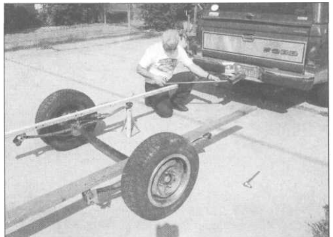
9.4 Bolt your springs, U-bolts, spring plates and shackles together, making sure the springs are square to the axle centerline and measuring the same distance apart front and rear.
