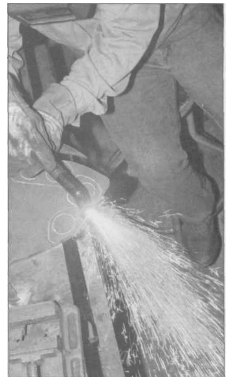
7.26 The 50-amp plasma cutter makes short work of cutting out the patterns and can easily pierce the center of a pattern to cut out internal holes and shapes.
