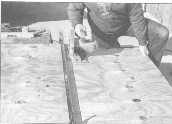
9.28 Having metal around for welding projects can pay off when working with wood, too. Use an extra length of straight angle-iron or tubing to clamp down on a piece of plywood as a saw guide, for perfectly straight cuts.
