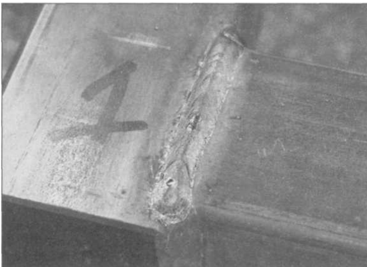
5.43 The tip-to-work distance is very important in maintaining the short-circuit arc. When practicing, watch the arc closely. The white-hot, melting end of the wire should stay about the same short distance from the puddle. Wire speed and welding travel speed control this.
