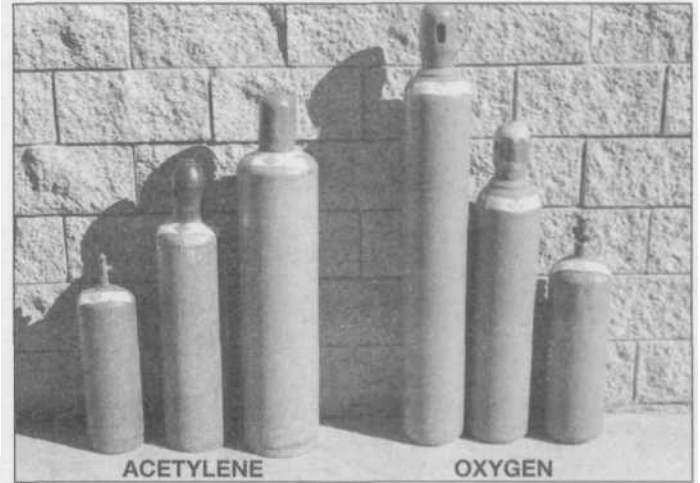
3.18 The small, medium and large welding cylinders contain 80, 150 and 275 cubic feet of gas, but some manufacturers label theirs by a letter designation. Ask your welding supply shop approximately how long each size would last in terms of welding, and choose according to your needs.
