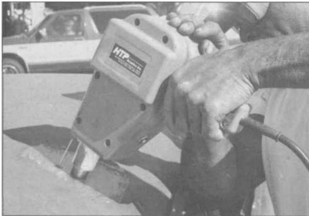
8.35 On a dented area that has been ground to clean metal, the tool is pushed in contact with the metal and the trigger is pulled for a half-second.
