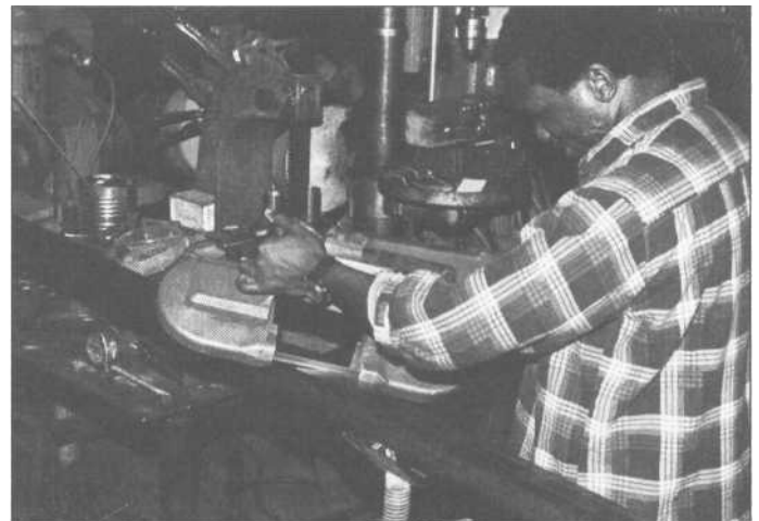
9.14 You can cut tubing and angle-stock with a hacksaw, but it is tedious. We borrowed a Milwaukee Port-A-Band hand-held bandsaw that made short, accurate work of fitting our tubing.
