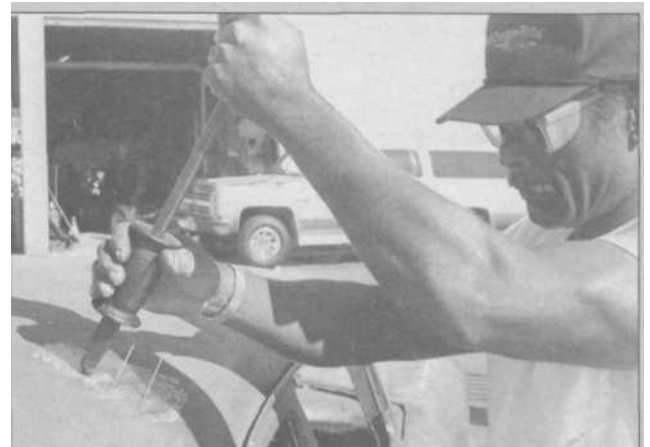
8.36 The studs are spot-welded in place, and a special slide hammer is used to pull out the dent or crease. Studs hold 500 pounds of pull.
